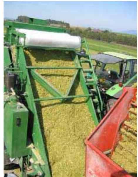
If the machine is running, the operator has nearly nothing to do anymore. All functions can be checked on the control panel, f. ex. speed of all conveying elements, chamber pressure or wrapping speed. If an error arises or the film or net tears, the whole machine stops. After the error is repaired, the automatic operation can easily be started again.
